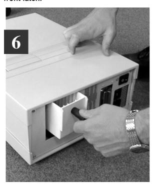
Install the Cassette into the printer from the rear.
